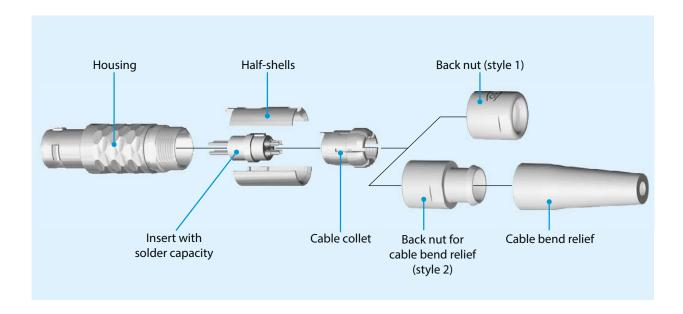
1. Slide back nut and cable collet (and possibly cable bend relief) over the cable.
