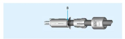
7. Now you can put the assembled cable considering the guidings (C) into the connector housing. If necessary, secure thread (D) with adhesive (see page 18).
