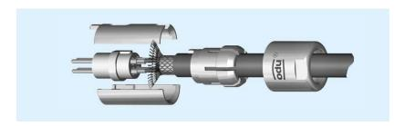
Slide the cable collet against the half-shells and clamp the shield (B) between it.
