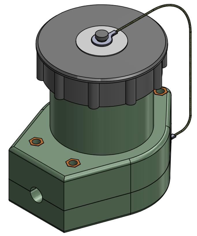
Place Bead of waterproof silicone adhesive on the bottom cap prior to assembly as show in picture to left.
